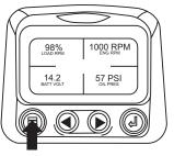
The main menu will pop up on the display. Use the "Arrow Buttons" to scroll through the menu until "Adjust Contrast" is highlighted.
